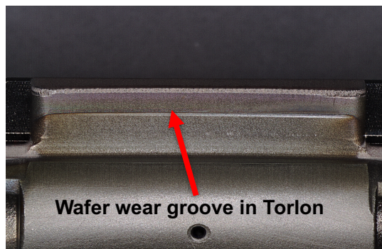
Fig. 7. VR optical image of wafer mark on Torlon fence after >350,000 wafer moves on disk. The mark is visually distinct under laser illumination but has very little depth, (see Fig. 8).
